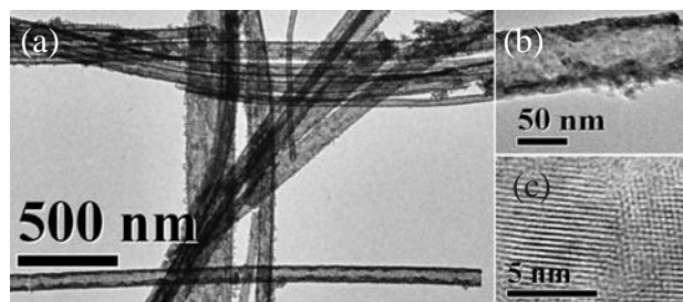
Figure 4. (a) TEM micrograph of CdS nanotubes, (b) TEM micrograph of a single nanotube with an open end, and (c) HRTEM image.
